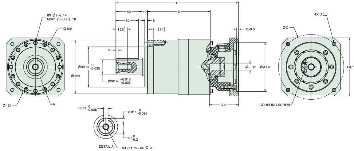
(Note) The dimension tolerances that are not specified vary depending on the manufacturing method. Please check the confirmation drawing or contact us for dimension tolerances not shown on the drawing above. Output shaft configuration shown is J6 (with a key and center tapped hole). J8 configuration has no key.
