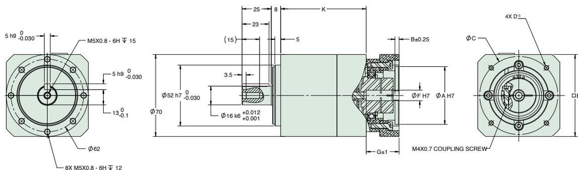
(Note) The dimension tolerances that are not specified vary depending on the manufacturing method. Please check the confirmation drawing or contact us for dimension tolerances not shown on the drawing above. Output shaft configuration shown is J6 (with a key and center tapped hole). J8 configuration has no key.
