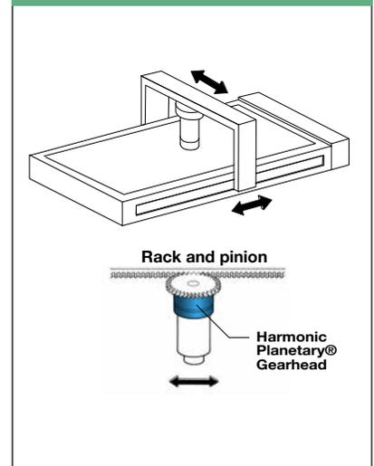
HPN-L Series Harmonic Planetary® High-Performance Gearhead for Servomotors
